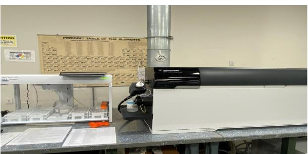
To further analyze the lead concentrations in Newark, NJ the water samples are going to be tested using a newer ICP-MS instrument model that can measure the concentration of lead in parts per trillion. For this ICP-MS we also need to create a calibration curve of standards of known concentration of lead. Prepared the following standards using a 1000ppm stock standard lead solution. All dilutions were prepared in 5% HNO<sub>3</sub>. Prepared a 1ppm and10ppb Solution as follows:
